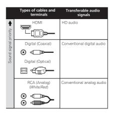
With an HDMI cable, video and audio signals can be transferred in high quality over a single cable.
